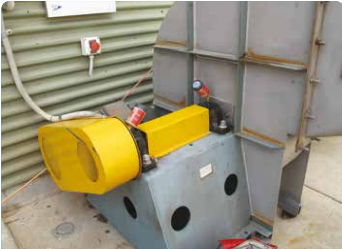
Application Fan support bearings Lubricator perma FLEX125 Installation kit Direct mount
