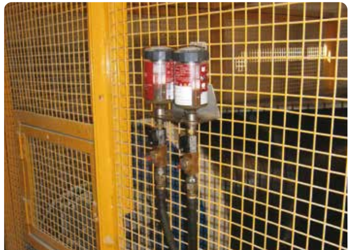
Application Conveyor pulley bearing Lubricator perma FLEX Installation kit K2CHG
